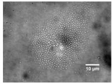
Researchers have demonstrated a new technology that combines a laser and electric fields to create engineering. tiny centrifuge-like whirlpools to separate particles and microbes by size, a potential lab-on-a-chip system for medicine and research. Here the technique is used to collect a bacterium called Shewanella oneidensis. (Purdue University image) **Download Photo**
