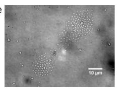
Here the rapid electrokinetic patterning technique is used to arrange bacteria into a specific pattern. The technique may be used as a tool for nanomanufacturing because it shows promise for the assembly of suspended particles, called colloids. The objects with colloids makes it possible to create structures with particular mechanical and thermal characteristics to manufacture electronic devices and tiny mechanical parts. (Purdue University image) **Download Photo**
