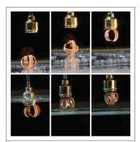
The graspers were coated with magnetic particles, which could allow researchers to retrieve the devices in the field by using a magnet. (Manuel Ochoa, Purdue University) A laser was used to machine the tape to a tenth of its original thickness, enhancing this curling action. The researchers coated the graspers with magnetic nanoparticles so that they could be collected with a magnet.
