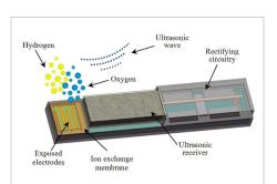
This diagram shows the design of a miniature device that can be implanted in tumors to generate oxygen, boosting the killing power of radiation and chemotherapy. (Birck Nanotechnology Center, Purdue University)
