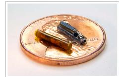
Researchers have created and tested a miniature device, seen here, that can be implanted in tumors to generate oxygen, boosting the killing power of radiation and chemotherapy. The technology is designed to treat solid tumors that are hypoxic at the center, meaning the core contains low oxygen levels. The device (right) fits inside a tube (left) that can then be inserted into a tumor with a biopsy needle. (Birck Nanotechnology Center, Purdue University)
